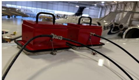
ARTS 7000 GPS couplers covering dual aircraft antennae.
